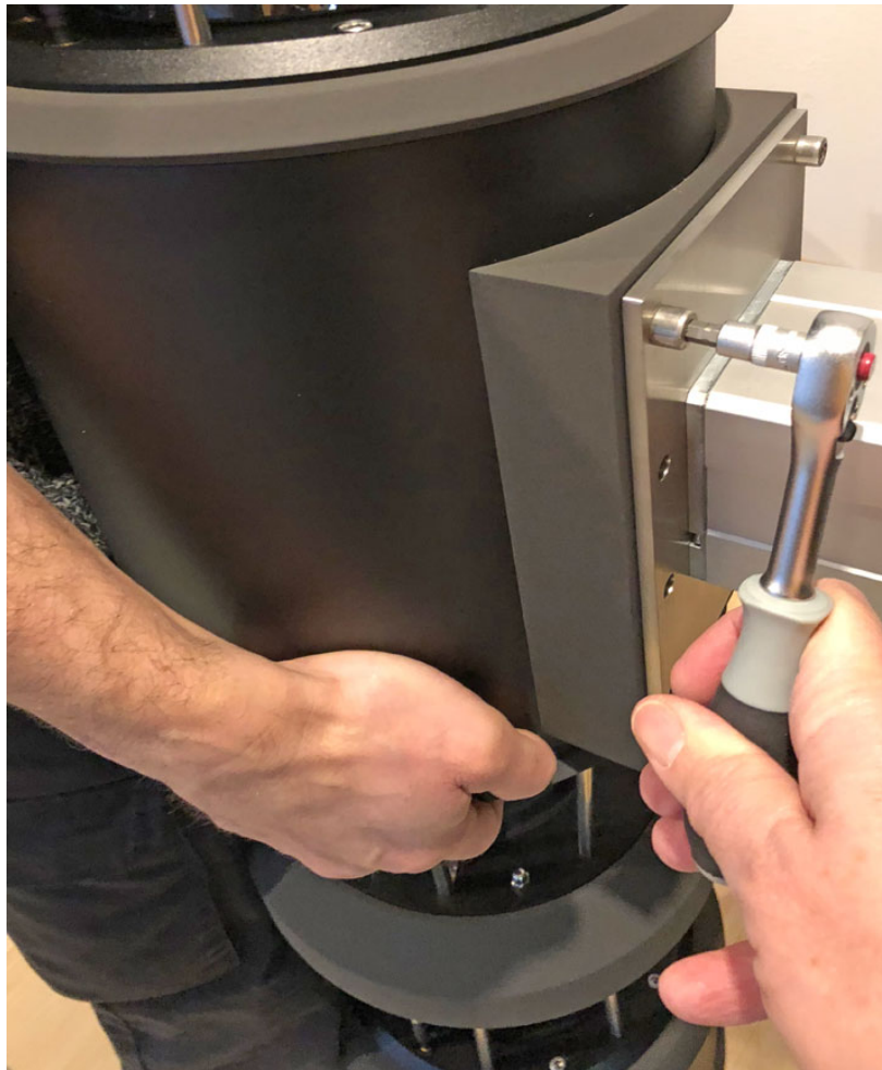
Figure 27. Fitting the DDD driver section.
