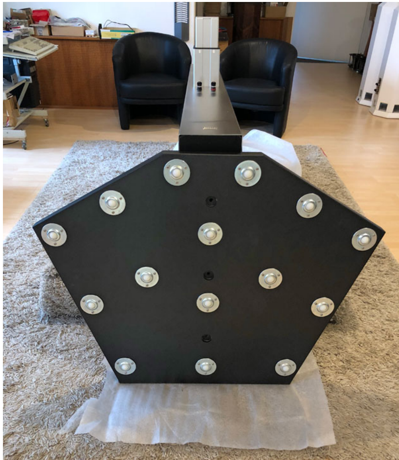
Figure 4. Offering up base plate to centre section.
