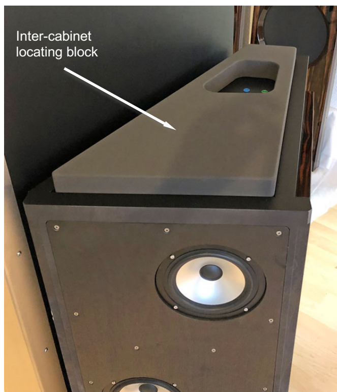
Figure 10. Inter-cabinet locating block.
