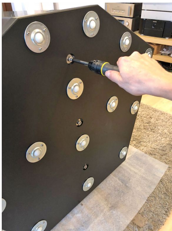
Figure 5. Tightening the base plate screws.
