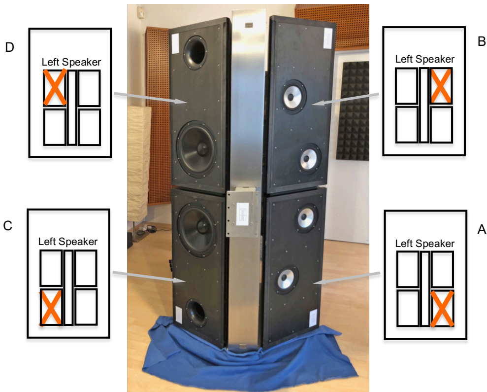
Figure 8. Bass cabinet identification labels for left loudspeaker.
