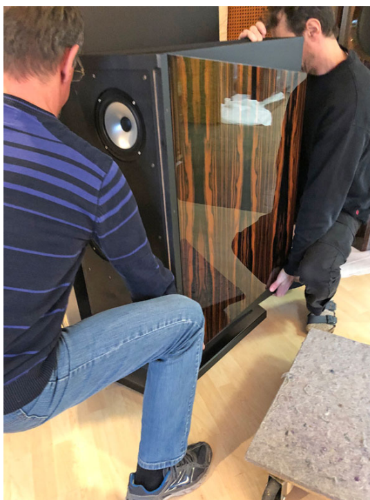
Figure 9. Fitting the left loudspeaker lower woofer cabinet.
