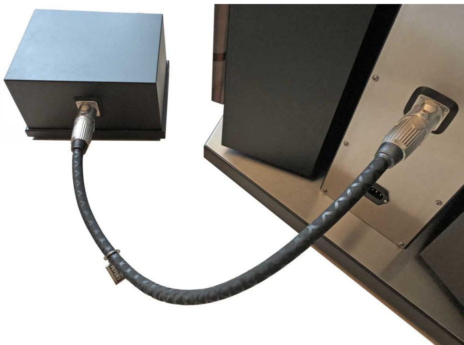
Figure 6. Amplifier connection box and umbilical cable.
